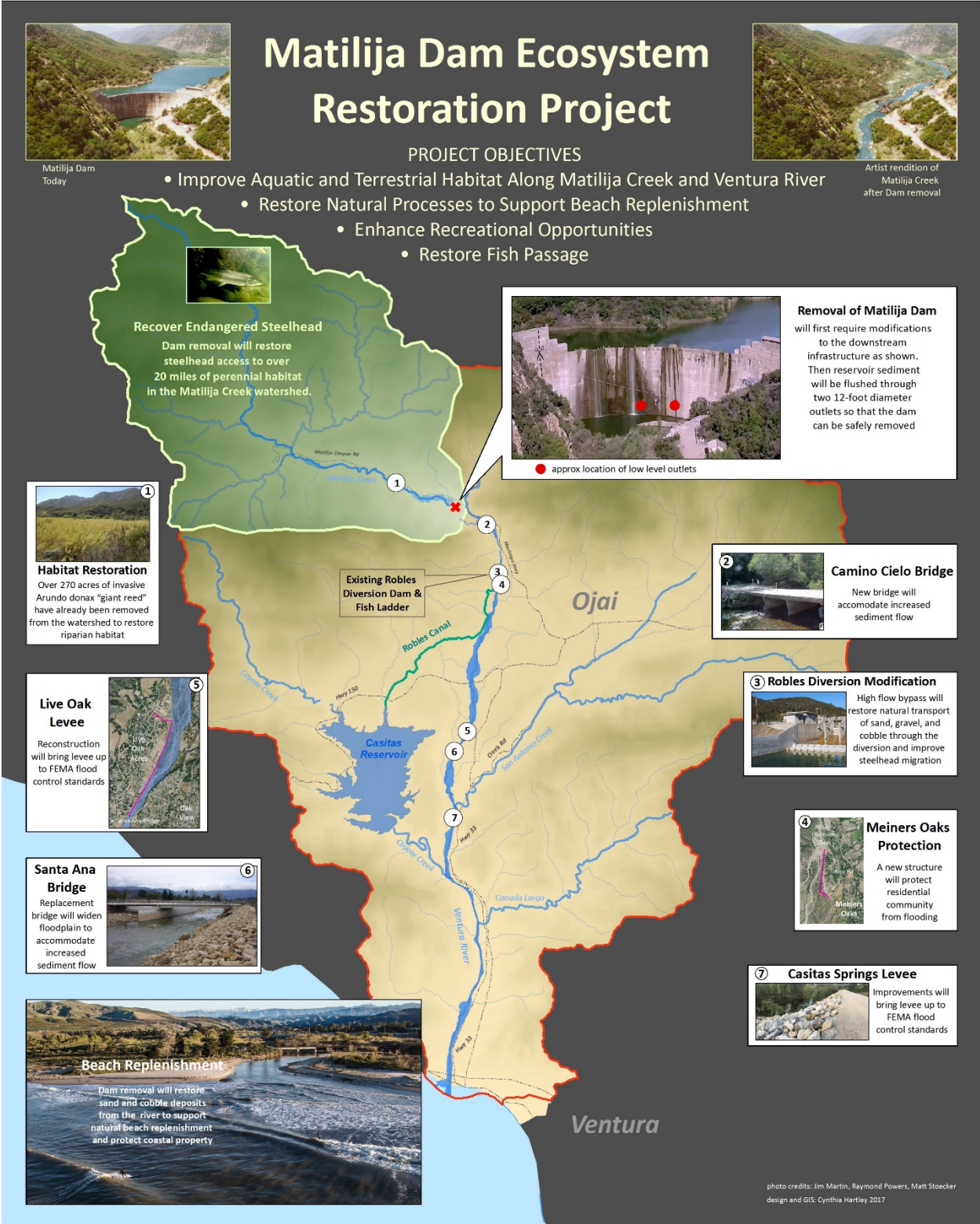
Figure 1: Matilija Dam Ecosystem Restoration Project Components
