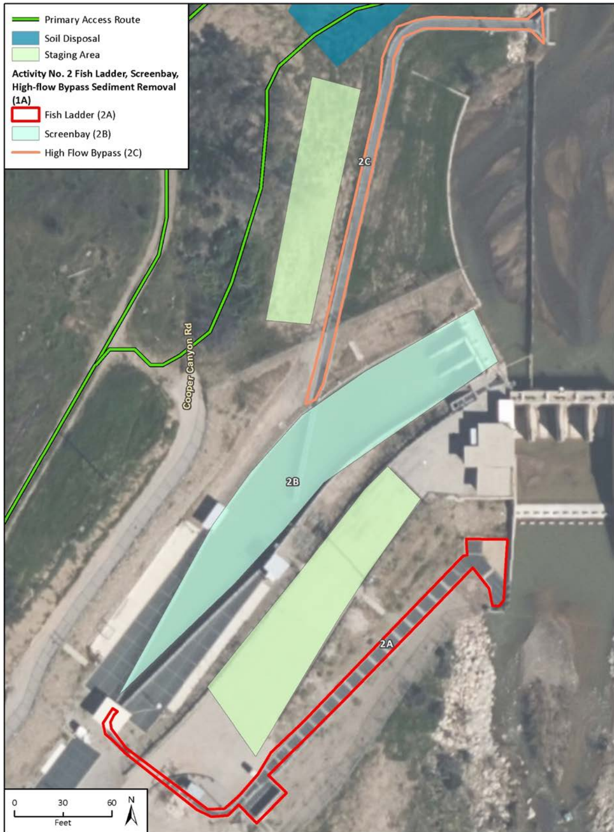
Figure 4 Activity 2 Fish Ladder, Screenbay, High-flow Bypass
